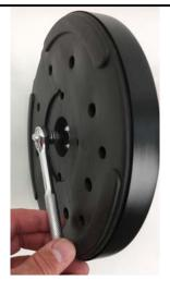
Using the 12mm socket & rachet, tighten the bolt while holding the pole with one hand.
