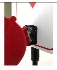
The Ticket Dispenser had two posts on the back of the unit that snap into the two holes in the mounting bracket. Line up the bottom post to the bottom hole and lift up/push back on the dispenser and it will snap into place. 6.
