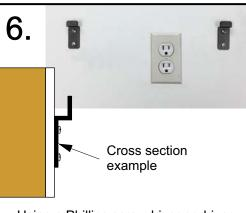
Using a Phillips screwdriver or driver bit and drill, mount the BRG EasyMount brackets utilizing the four screws that were provided in the hardware bag into the plastic keepers. Tighten the screws.
